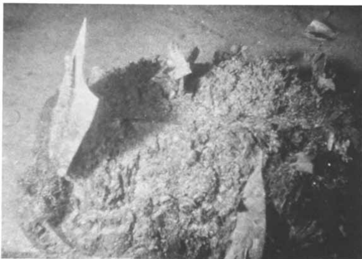
Figure 1. A 15–20-kg waste bale after immersion for about 11 months at 15 m. This bale was not meshed, and there has been no benthic organism attachment except on straps.
