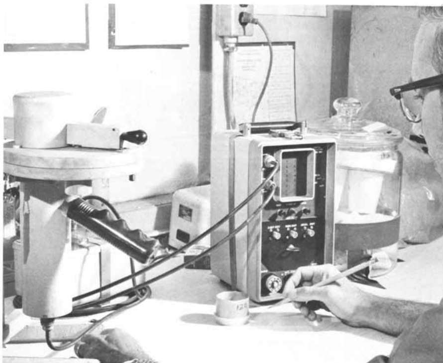
Figure 4. A view of the x-ray fluorescence apparatus used onboard the R/V Prospector for nodule analysis
