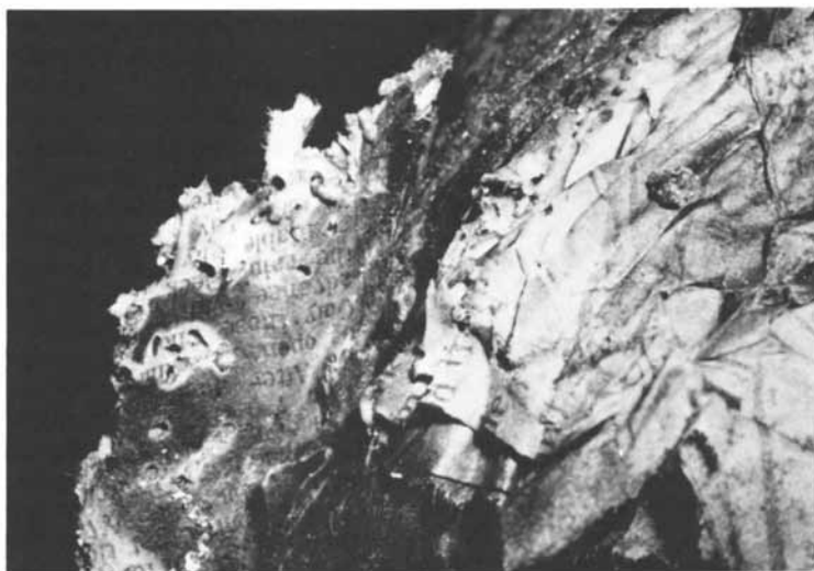
Figure 4. Photograph of newspaper from the outside 10 cm of an experimental waste bale immersed for 13 months at 15 m. The burrows on the left were found in the outside 2–4 cm and were made by a burrowing isopod Limnora ligorum . The dark areas are due to precipitation of iron sulfides.
